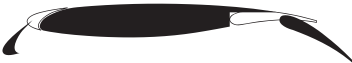
Figure 1. The MDC 30P/30N configuration with deployed slat (forward) and flap (aft) components.
